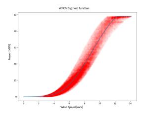
Fig. 5: Wind-Power Conversion Model
